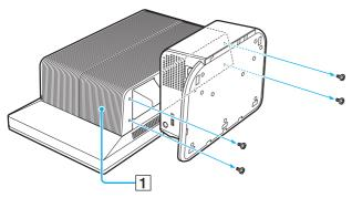
5 Slide the back panel toward the bottom of the computer, lift the panel, and set it aside.
